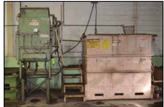
Hydraulic Reclaiming / Separation Unit & Holding Tank
