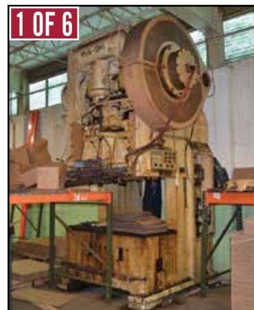
(6) BLISS 176-B 115-Ton Gap Frame Presses
